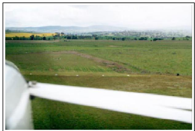
**Picture 1 & 2.** This is what you may see if the rope has broken at a rather low height, travelling south west, down the hill on the main strip. The white parts in the photo are the struts of the tug. There are a couple of fences almost invisible to you, just in an area where you might consider putting it down.
